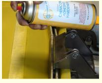
**Step 3.** Apply ChemCon Adhesive Hardener, aerosol or liquid directly over the adhesive
